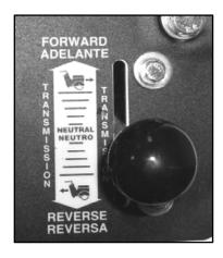
Figure 19: Speed Control Lever
